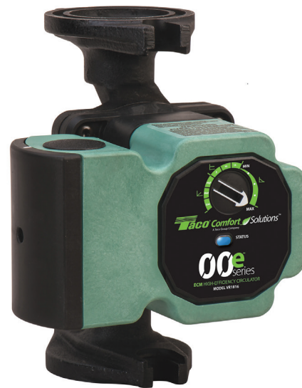
Taco's ECM wet rotor 00e VR1816 circulator offers up to 18 feet shut-off head and 16 gpm flow.
