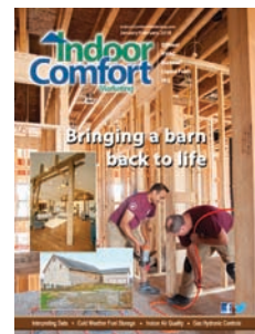
Cover: Man Khadka, installer (left), and Vince Youndt, owner, Vertex Mechanical, connect 1/2-inch Watts Radiant PEX+ tubing to the home's upstairs subfloor. Watts Radiant photo by John Herr
