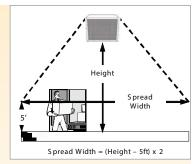
than recommended can result in complaints of low heat output. Mounting a unit too low can result in complaints of too much heat.
