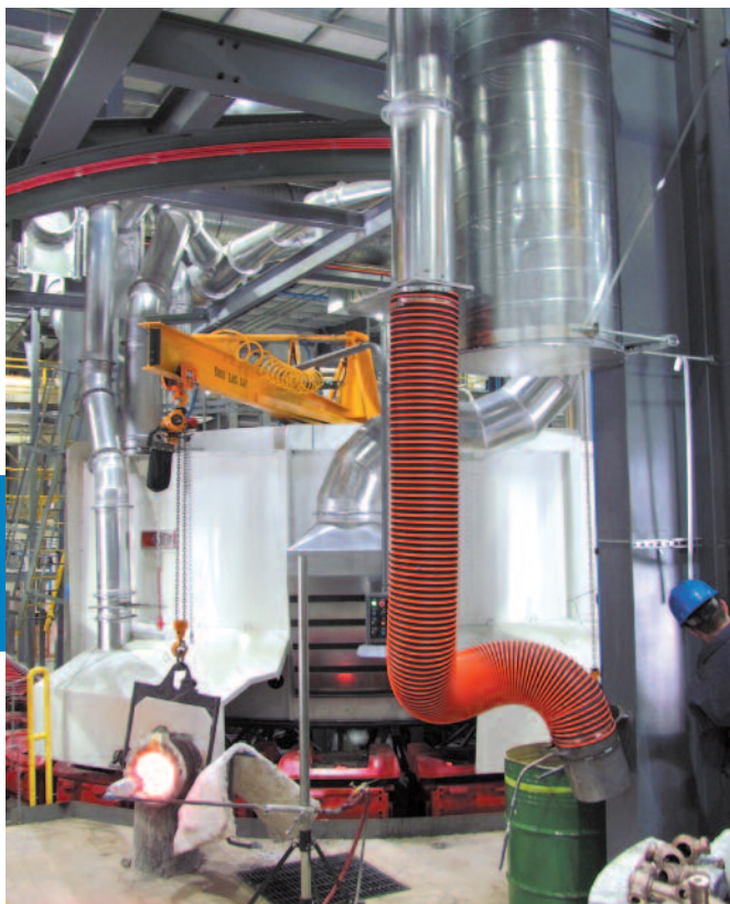
Heating a crucible prior to pouring molten bronze into molds.
