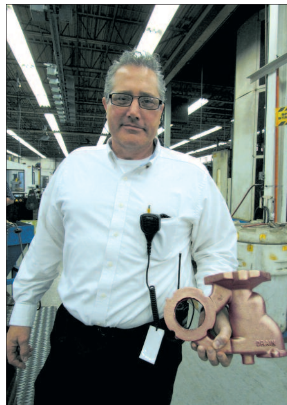
Director of Operations Tyler Stone shows off one of the lead free castings made at Watts' new foundry.
