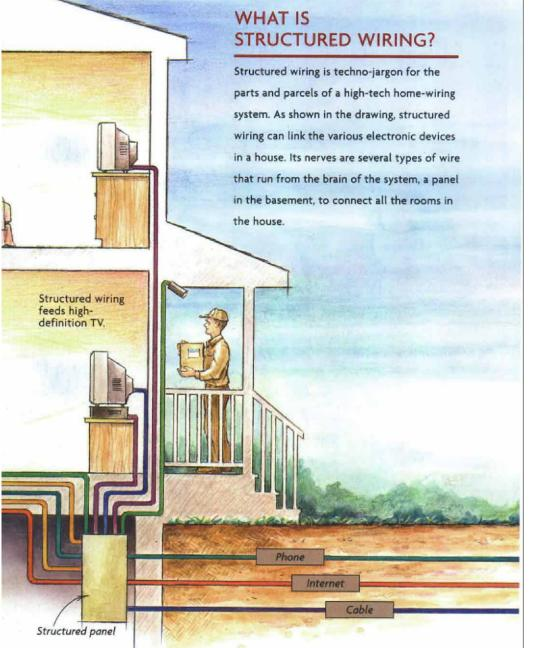
than turbocharged phone wire and coaxial cable. My company installs miles of the stuff. The biggest factor to keeping down installation costs is to get the wiring in before drywall goes up. The cost of doing a structuredwiring system later can be up to four times the cost of installation while the home is under construction.
