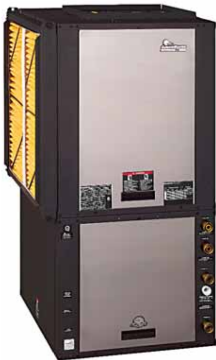
ClimateMaster's HFC-410A Tranquility 27 water-to-air geothermal heat pumps extend from 2- to 6-ton sizes with efficiencies up to 31.5 EER and 5.1 COP in upflow, downflow, horizontal and split system configurations.
