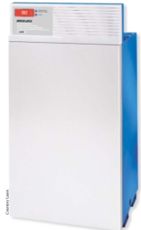
Counter-flow design preheats cool return water before it reaches the inner jacket in the boiler at left. Above, this boiler uses automatic burner modulation ranging from 57 percent to full fire, preventing short cycling.
