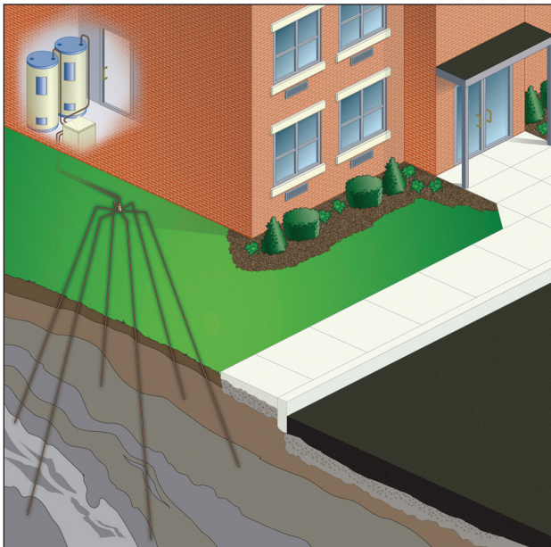
The EarthLinked system pre-heats water before it enters the holding tank.
