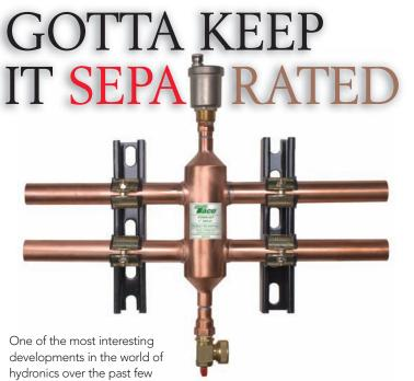
years has been hydraulic or "hydro" separators. Also known as low-loss hydronic headers, these components create a low-pressure zone, enabling the connected primary and secondary loops to be hydraulically independent.
