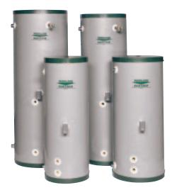
cleanings. Domestic hot water is stored in a heavy-duty 316L stainless-steel tank. Two-inch foam insulation keeps the water hot with a standby loss of less than <sup>1</sup>/2°F per hour. These units come equipped with an adjustable, well-type Honeywell control and a T&P relief valve as standard equipment. Peerless indirects are available in 37-, 57-, 77-, and 119-gallon sizes.
