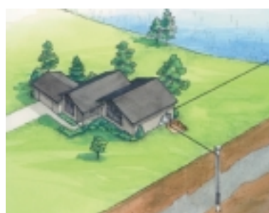
Closed-loop geothermal water source systems (top and middle) use continuous loops of buried plastic tubing as a heat exchanger. Open-source systems (bottom) use ground water as a direct energy source for home heating and cooling.
