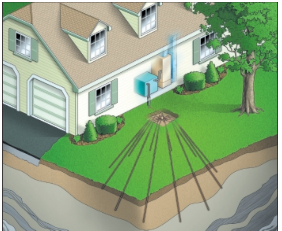
Basic diagonal earth loop system.
