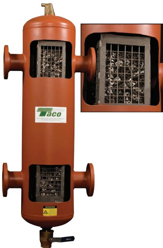
**The FlexBalance hydraulic balancer from Taco acts as a hydraulic bridge between the primary and secondary circuits in hydronic heating and cooling applications. The 5900 Plus model uses a Pall ring assembly that removes gases from water.**
